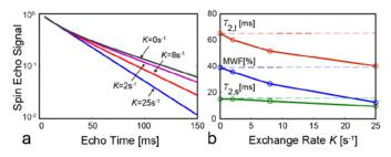
Fig. 4. Dependence of spin echo signal (a) and apparent MWF and  $T_2$  values (b) on the exchange rate *K*. In (b), the dashed lines show true parameter values and markers correspond to *K* values from (a). The deviations of signal and parameter values grow with the exchange rate.
