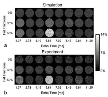
Fig. 9. MTR in fat+agar phantoms at different echo times calculated by simulation (a) and measured at 3.0T (b). Note significant variability of MTR with fat fraction and echo time.
