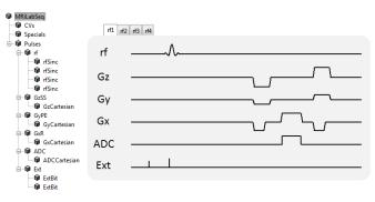
Fig. 2. An example of a hierarchical balanced steady state precession (bSSFP) sequence tree structure with the corresponding generated waveforms. Four separate RF sources in the tree permit modeling of parallel RF transmission (for display purposes, only one RF source within one TR is shown). The pulse sequence is built from tunable macros which provide modularization and reusability.
