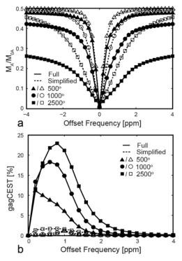
Fig. 8. Comparison of gagCEST simulations using simplified (two non-exchanging pools, dashed lines) and full (three exchanging pools, solid lines) models. (a) gagCEST Z-spectra and (b) the asymmetry plots simulated for simplified and full models for several off-resonance saturation powers ( $\alpha_{CEST}$ =500°, 1000°, 2500°).
