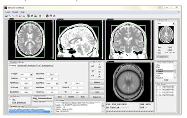
Figure 1. 3D-bSSFP simulation at 3.0T using MRiLab. Figure shows the main simulation panel and one axial slice of simulated bSSFP image. Note banding artifact is caused by added field variation.
